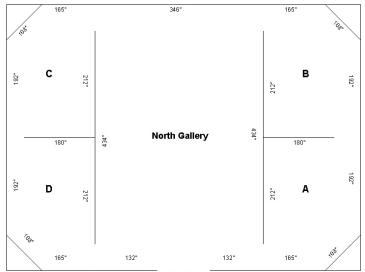
Outer walls of gallery: approx 26' high, made of sheet rock, plywood and concrete inner partitions: 12' high, made of sheet rock and plywood
